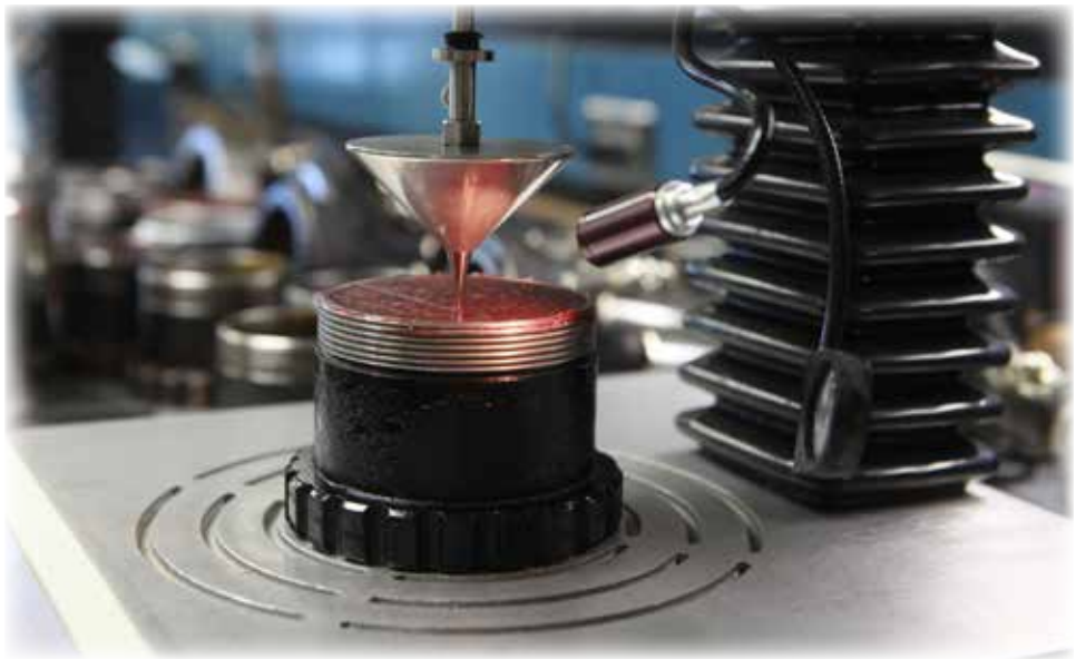
The ASTM Cone Penetration Test, which determines consistency, is the primary quality control test for lubricating greases. This test is performed on every grease processed at the LE manufacturing facility and is used to determine the NLGI grade.
