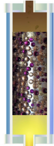
Acid levels lowered, Resistivity increased, metals and varnish molecules removed
