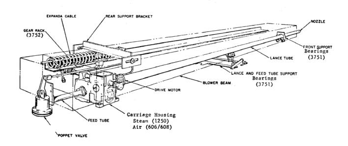
All are ruggedly built, to operate dependably on both indoor and outdoor boiler tower installations. Swirling of the blowing medium gives maximum cooling effect on the lance, which lends to long service life in almost any furnace temperature.
