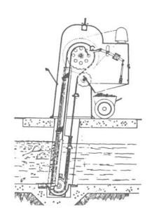
On the traveling screens, each section must be thoroughly lubricated to allow movement without binding. Since the sections move through the influent stream, they must be lubricated with water-resistant grease such as LE's 3750 - 3752 ALMAGARD® Vari-Purpose Lubricants, LE's 1275 ALMAPLEX® Industrial Lubricant, LE's 9901 ALMASOL® SYNTEMP® Lubricant or LE's 5182 PYROSHIELD®.
