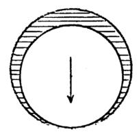
B - When the journal starts to rotate, it tends to move up the slope of the bearing.
